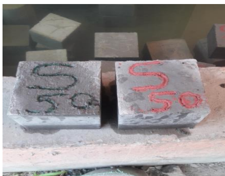
Figure 7 : WMCA replaced cubes out of mould for testing
