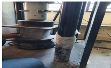
Figure 8 : Cube placed in CTM for loading
