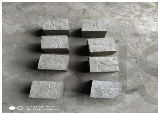
Figure 6 : Standard cubes removed from mould for testing
