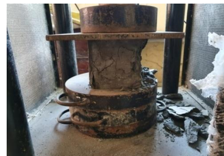
Figure 9 : Cube specimen after failure
